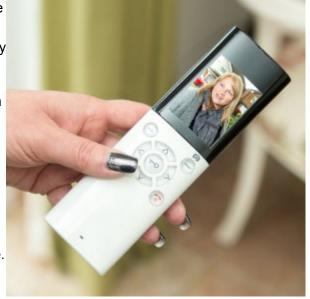
communication, others are two-way, allowing full conversation. Some have a handset which must be used when speaking through the system, others have a hands-free facility. This may allow the unit to transmit messages once speech is sensed. If no speech is sensed, the unit remains on receive mode.
