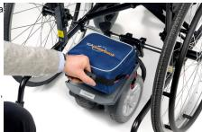
Depending on the drive mechanism, some units required particular wheels to be fitted to your chair and some require an anti-tipping mechanism adding.
