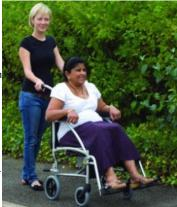
Self-propelled chairs have large rear wheels for the user to grasp and push. Attendant-propelled chairs have much smaller rear wheels. This
